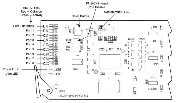
Figure 2-5. DNH-6800 Board Graphic Showing Indicators and Controls
